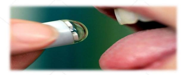
It is basically a multichannel sensor used for remote biomedical measurements using micro technology. This is used for the real-time measurement parameters such as temperature, pH, conductivity and dissolved oxygen. The sensors are fabricated using electronic beam.
